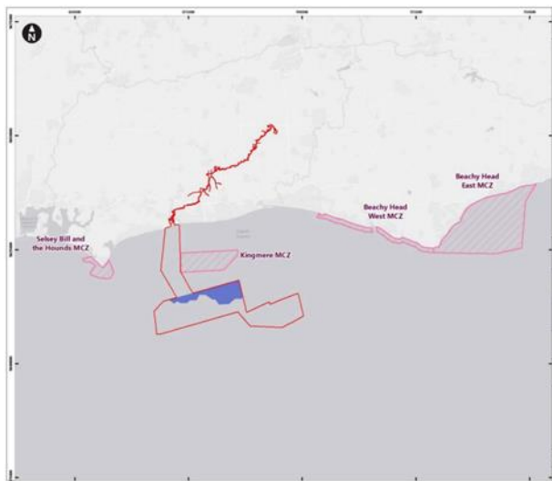
Figure H-3 Piling exclusion zone for the piling of multileg foundations , with 20dB reduction ( Unwtd, 141dB SELss )
