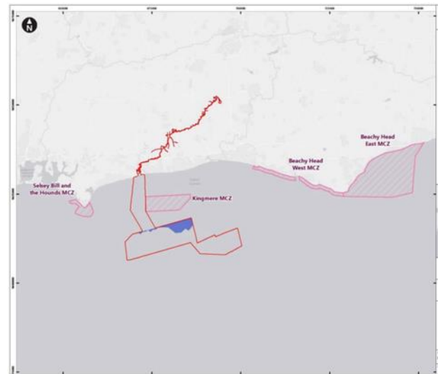
Figure H-4 Piling exclusion zone for the piling of multileg foundations , with 20dB reduction ( Unwtd, 141dB SELss )
